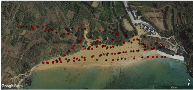
Figure 3: Drone flight plan during the survey. Red dots indicate the UAV position during the image acquisition.
